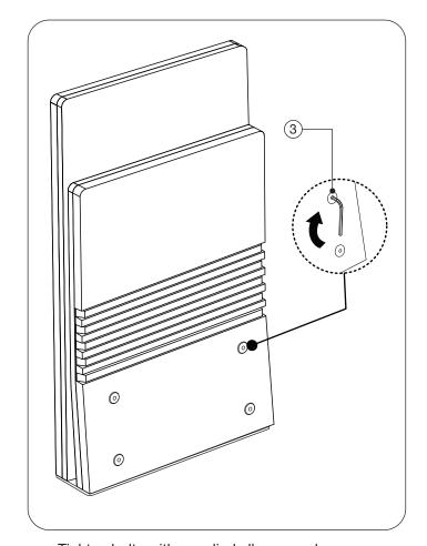
• Tighten bolts with supplied allen wrench.
