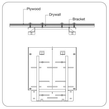
Mounting with Plywood Reinforced Drywall
