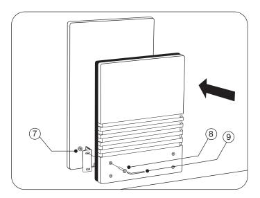
• Attach seat with 1/4-20 nuts and bolts, tighten with allen wrench.
