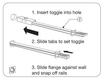
Installing the toggle anchors for drywall or cinder block walls.
