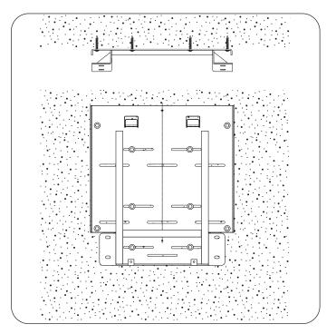
Mounting on Concrete Wall
